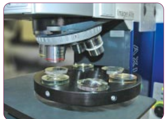
Central force sample holders feature a stable, low profile design allowing observation on an upright microscope (shown on a Zeiss AxioImager Microscope)
