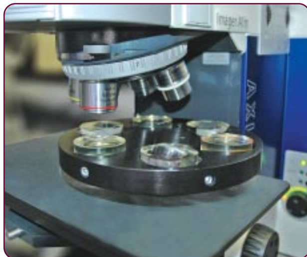
Central force sample holders feature a stable, low profile design allowing observation on an upright microscope (shown on a Zeiss Axiolmager Microscope)
